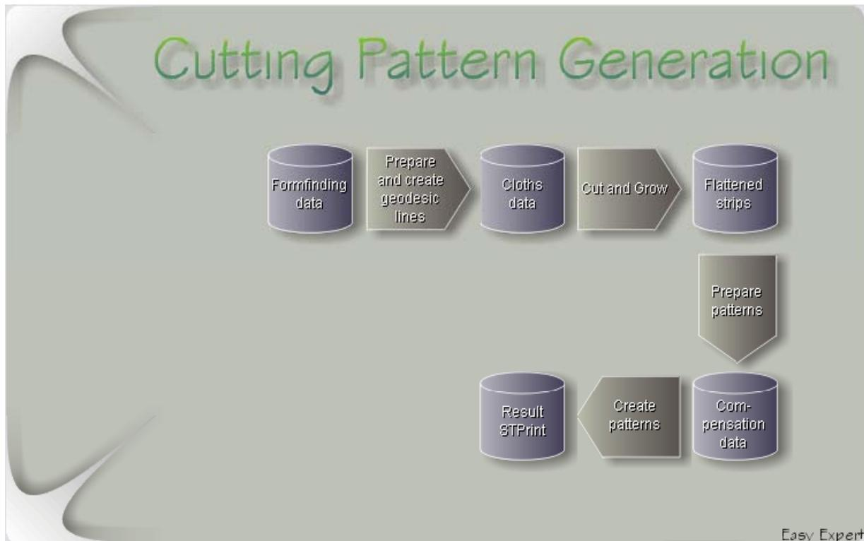
**Figure 13:** Diagram Easy Cutting Pattern Generation.
