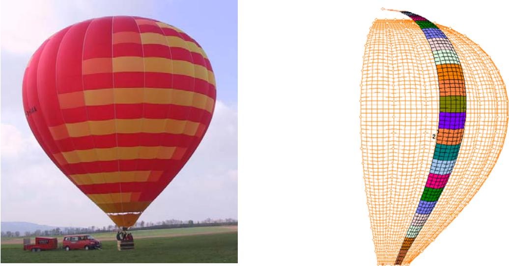
Figure 9: Formfinding and statical Analysis under inner pressure and bouyancy
